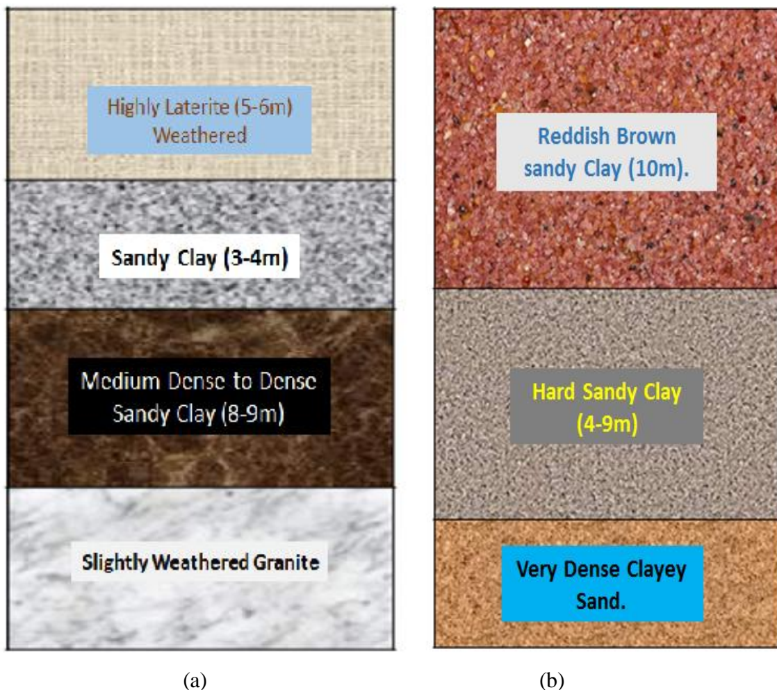
Figure 5: Soil Profile observed at Murudeshwar and Honnavara
